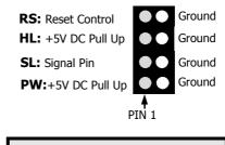
Top View of the System Panel and LED Connectors
